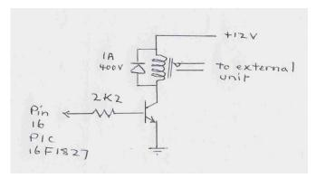
The choice of transistor is not especially critical providing it has a suitable current rating to drive the relay. Because the relay may be on for lengthy periods it may be necessary to heatsink the transistor.
