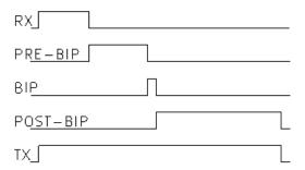
This diagram shows the relationship of the tail options. Pre-bip is the normal tail, while Post-bip is the extended tail. The timeout timer is reset when the RX COS drops out. The extended tail timer has multiple uses in the controller.
