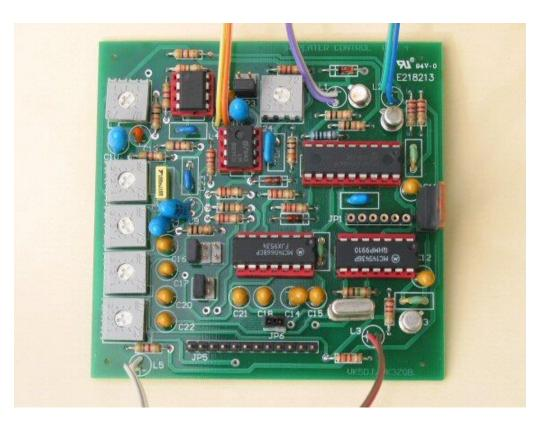
A design for a repeater controller for amateur or professional use. On a board 80mm by 82mm, the controller is a two port design intended to control a duplex repeater with or without a simplex gateway or link.
