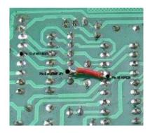
Install all the resistors but note positions of R21,R22. Solder to upper board and bottom trace where jumpers are required if you are not using a plated through board. I recommend mounting R21/R22 vertically with the resistor body against the board on the south side (see above for orientation). If you need to change COS polarity at a later date it is then easy to cut the resistor lead in its centre and bring a wire up from the alternate hole in the board.
